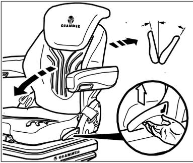
Pull up the locking lever to release the backrest catch. When releasing the backrest catch, do not apply load to the backrest by pressing against it.
