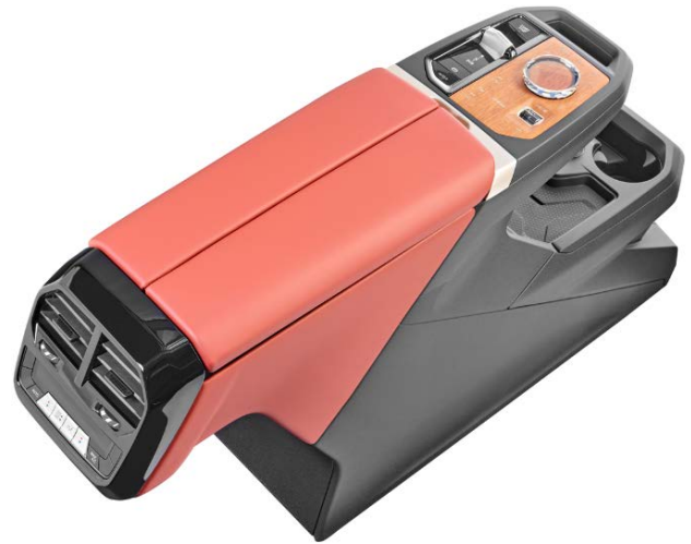
Free standing design of the center console in the BMW iX. Source: GRAMMER AG
