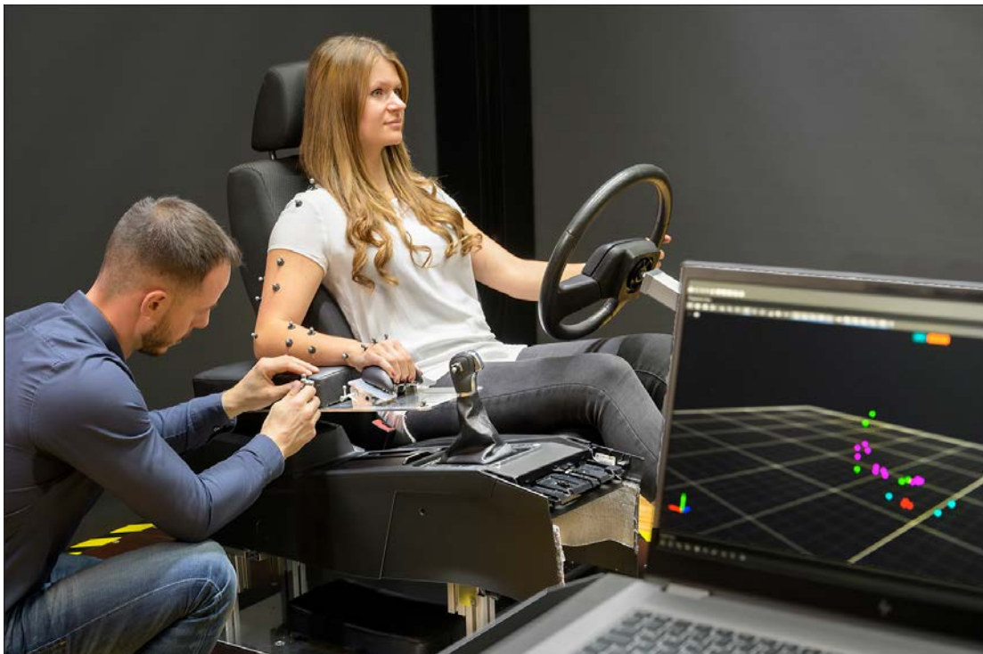
Focus on users: In the test cube of the Grammer ErgoLab, center consoles are evaluated in terms of ergonomics, haptics and operating comfort under a wide range of different lighting conditions. Source: GRAMMER AG
