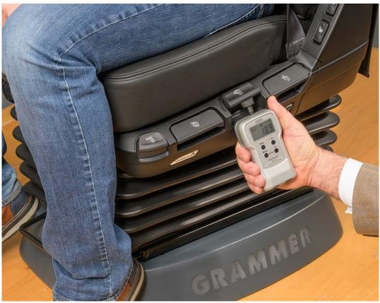
Highly accurate testing: Professional equipment is used to measure the operating force required for switches.
