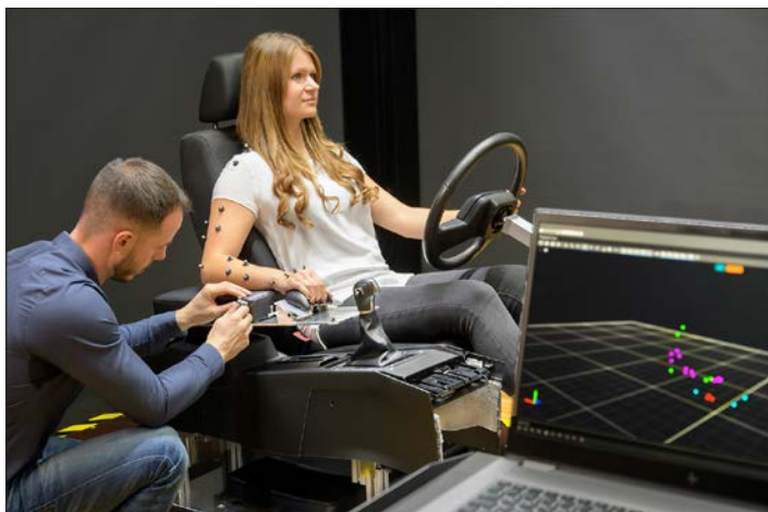
Focus on users: In the test cube of the Grammer ErgoLab, a motion capture camera system records user profiles - here in an automotive interior – for different interactions with seats and interior components.
