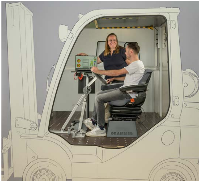
Comfort and ergonomics testing in the Grammer ErgoLab: Dr. Susanne Frohriep, R&D Senior Manager Global Ergonomics, Usability & Design talking to a test person in the cabin mockup of a forklift.
