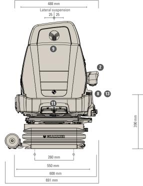
Measurements (installation dimensions)
