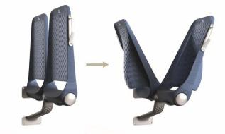
Can be used in both directions of travel without conversion: The new Ubility Light from Grammer offers many options for flexible configurations in buses, trains or autonomous shuttles.
