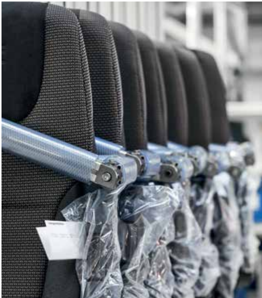
The backrests are ready for assembly of the base structure.
